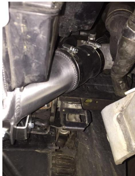
\*Note – Make certain there isn't any dust or debris inside the intercooler before fitting by giving it a shake or blow out with an air line.
