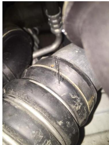
Next attach the silicone reducer to turbo outlet and tighten hose clip. You won't be able to reach this hose clip when the new intercooler is in so insure it's tight.
