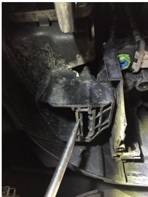
Attach the supplied bracket to the block using the provided nuts and bolts, making sure the bracket is mounted as shown below.
